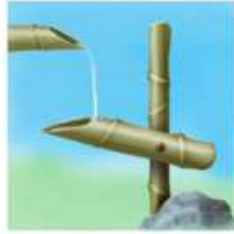
Full tube begins falling.
